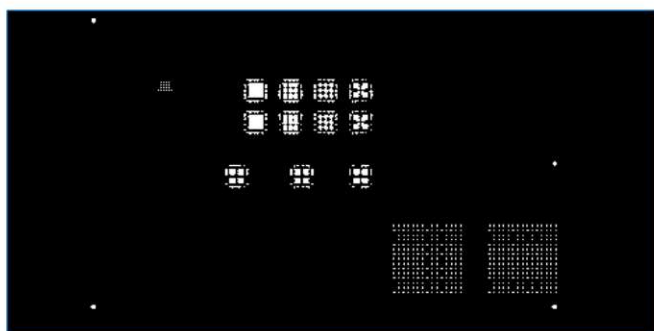
FIGURE 1. Layout of the test board with five different apertures for BTC components.
